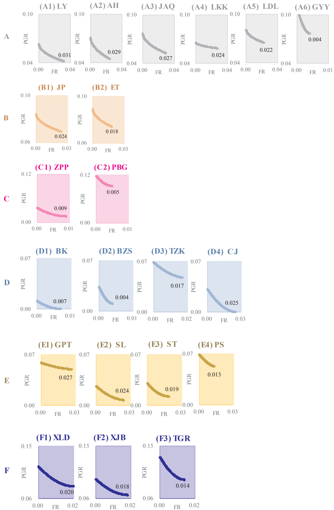
Fig. 6. Pareto Frontiers between flood risk (FR) and power generation risk (PGR). The illustration is made for 21 cascade reservoirs in six regions (A-F) of the whole Upper Yangtze River Basin.
