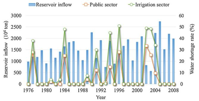
Fig. 4. Inflow of the Shihmen Reservoir and water shortage rates of irrigation and public sectors in the study area, respectively (1976–2008).
