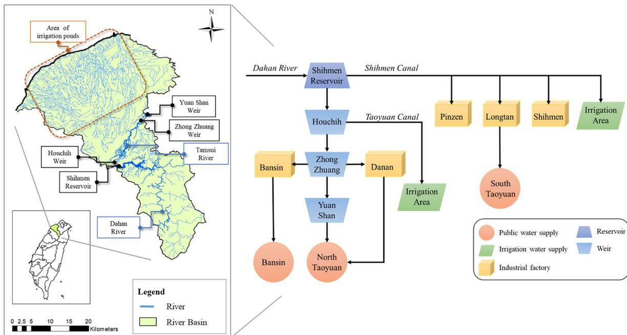
Fig. 3. Schematic diagram of the Shihmen Reservoir Water Supply System.
