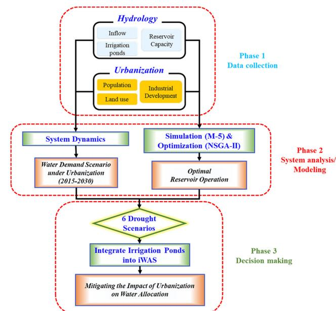
Fig. 1. Flow chart of the proposed intelligent water allocation system (IWAS) for apt water resources management under urbanization.
