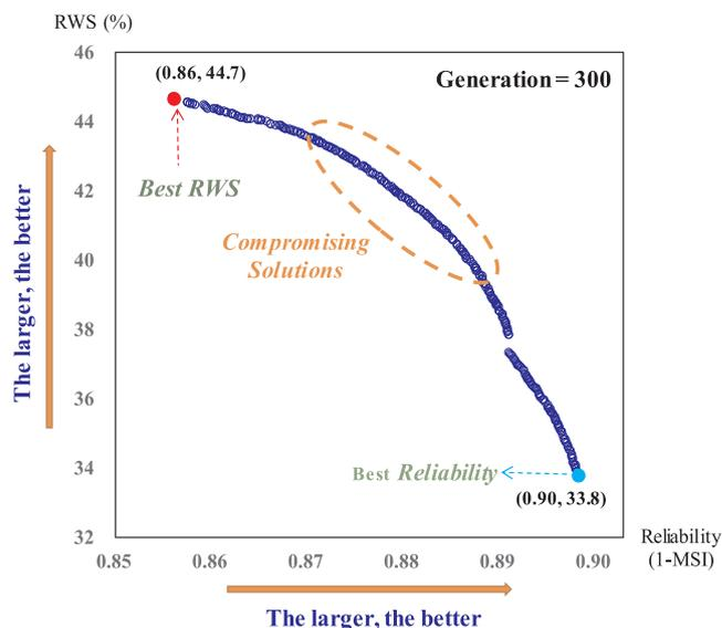
**Fig. 7.** Pareto Front of the NSGA-II with respect to the ration of water storage to reservoir capacity (RWS) and water supply reliability (=1-MSI) under the Scenario with reservoir inflow of year 2002 and initial reservoir storage capacity = 50% ( $S_{50\%}$ ), which converges at the 300<sup>th</sup> generation.
