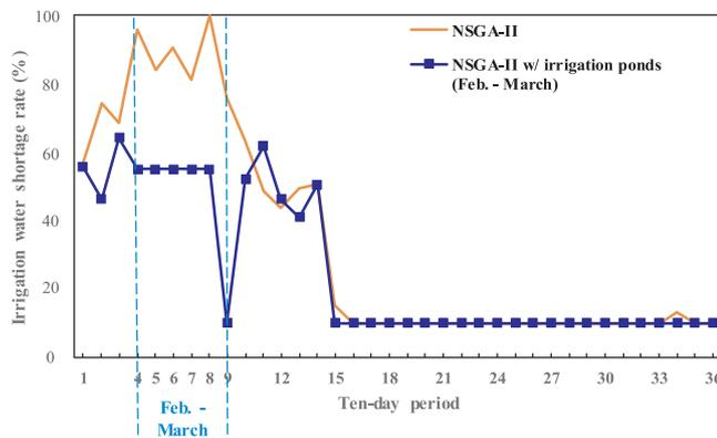
Fig. 8. Improvement of drought mitigation under the Scenario with reservoir inflow of year 1977 and initial reservoir storage capacity = 50% ( $S_{50\%}$ ).
