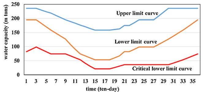
Fig. 5. M-5 operation rule curves of the Shihmen Reservoir.
